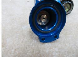
Use blue loc-tite on screws. Adjust the fuel pressure tighten the jamb nut and install vacuum line on the end of the lead screw,
